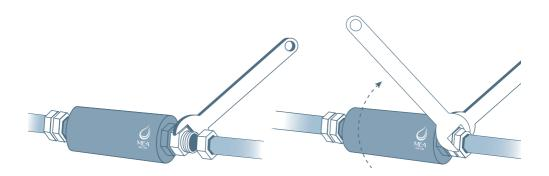
For operation to WaterMark Australia standards, installation must be in accordance with AS/NZS3500 and have a dual check valve (dcv) fitted between the water meter or pump and the device (see diagram). This product complies with the requirements of Lead Free standards as defined in the National Construction Code Volume 3 and is suitable for use as part of Lead Free installation.
